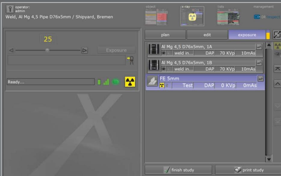
**OR**inspect fully controls your Golden Engineering generator. The software allows easy setting of the pulses and triggering of the exposure. All values e. g. pulses are preconfigurable.
