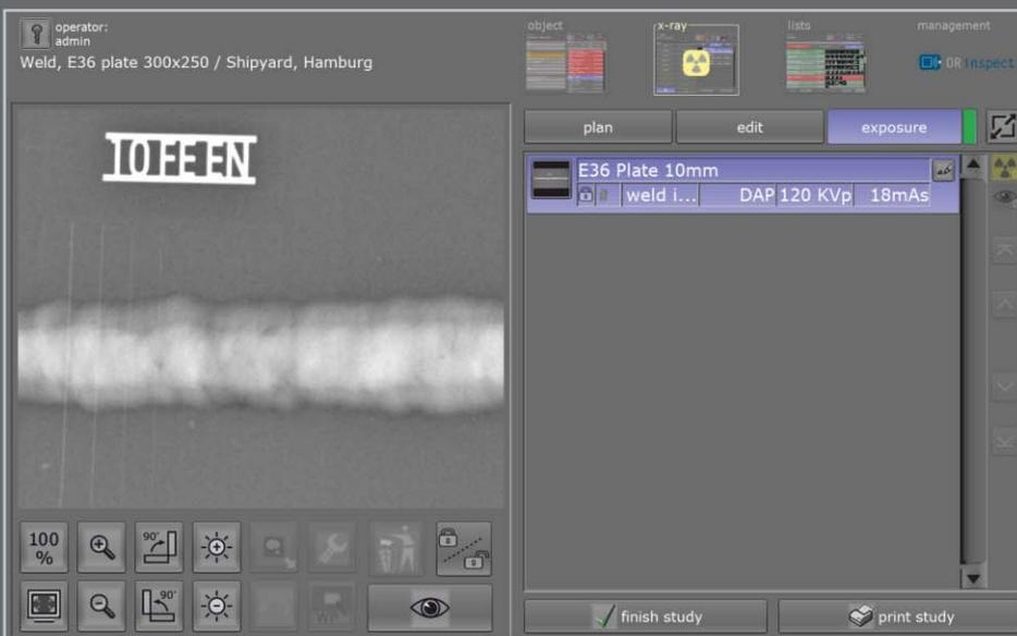
**OR**inspect provides a quick preview image of the inspected object. Easy access to important software tools e. g. for verifying the exposure or entering the internal viewer.
