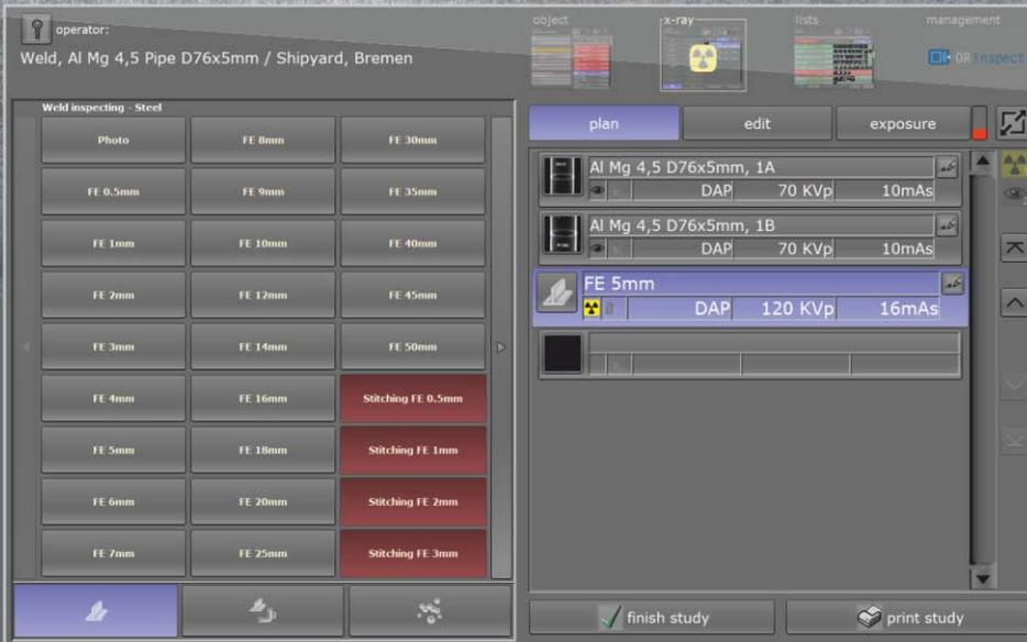
**OR**inspect provides pre-defined examinations that can be adapted to your recurrent inspection tasks. The software stores your individual examination/inspection values. Complex test procedures can be saved as macros.
